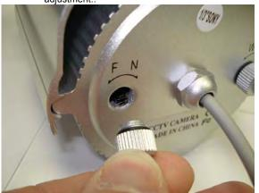
4. Then use a small standard screwdriver to adjust the focus of the camera.
